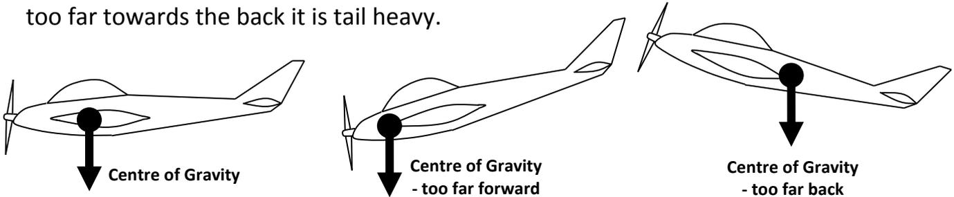
Prior to take-off the pilot must check that the aircraft's centre of gravity is within the recommended limits. If it is outside of the limits the aircraft may not be able to be controlled safely.
